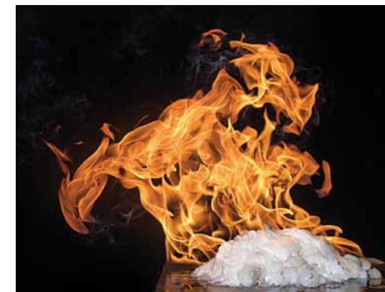
Gas hydrates are methane gas trapped inside cages of frozen water molecules.
